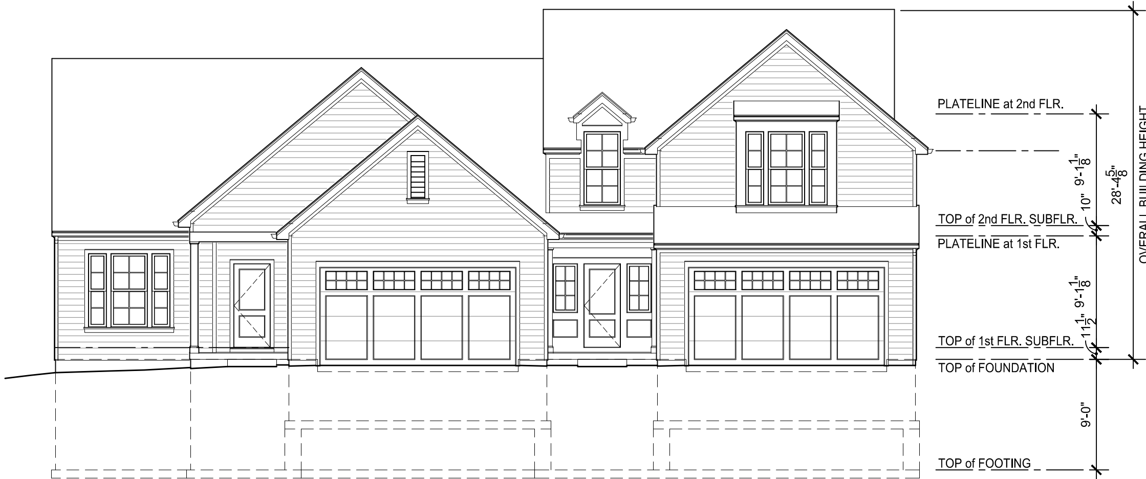
FRONT ELEVATION - TWIN VILLAS
