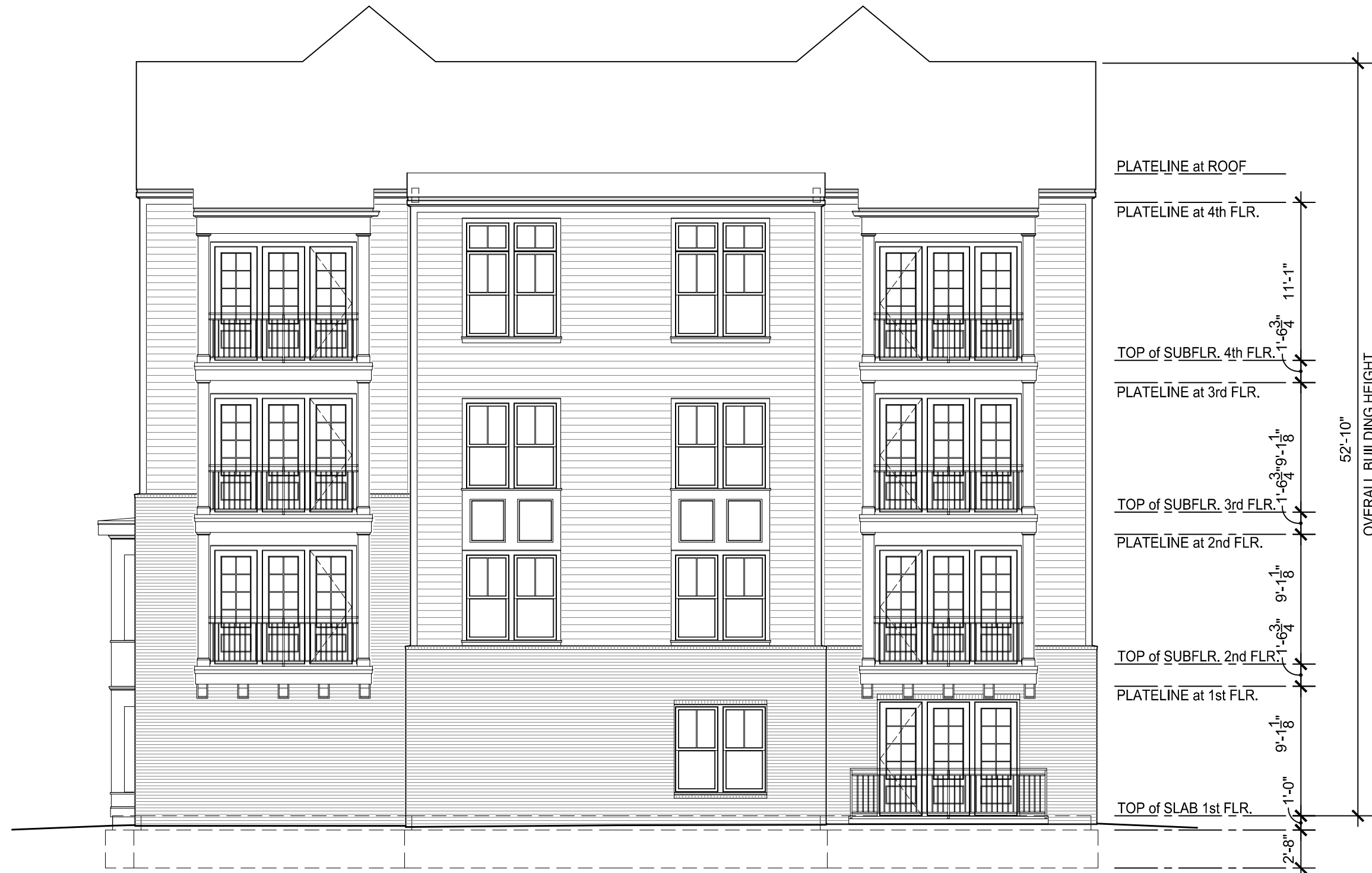
RIGHT SIDE ELEVATION - BUILDING 'B'
