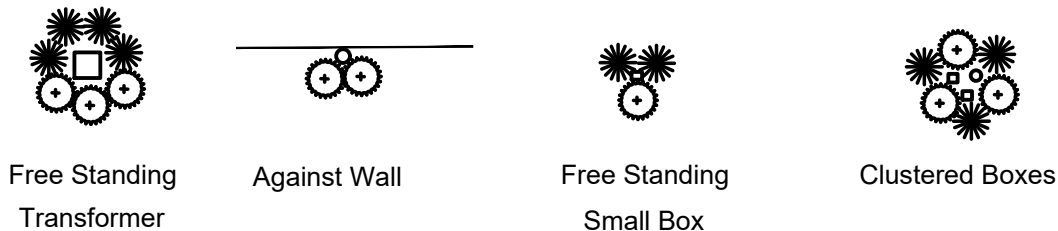
TYPICAL UTILITY BOX SCREENING DETAILS - NTS
