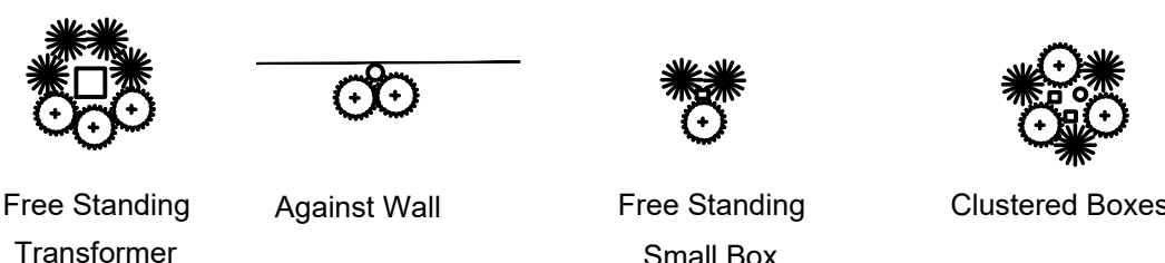
TYPICAL UTILITY BOX SCREENING DETAILS - NTS
