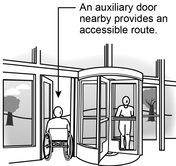
Auxiliary Door at Inaccessible Revolving Door
