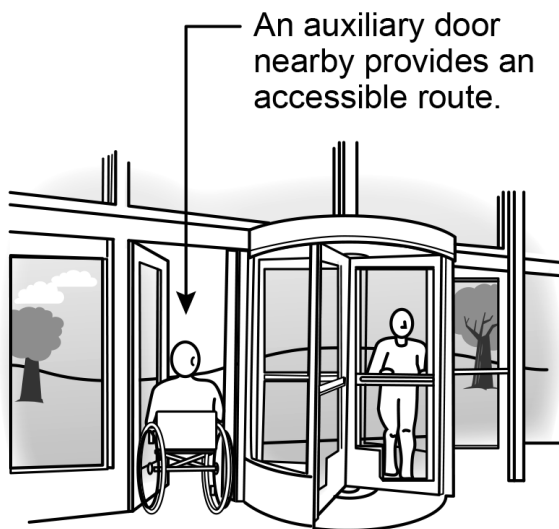
Auxiliary Door at Inaccessible Revolving Door
