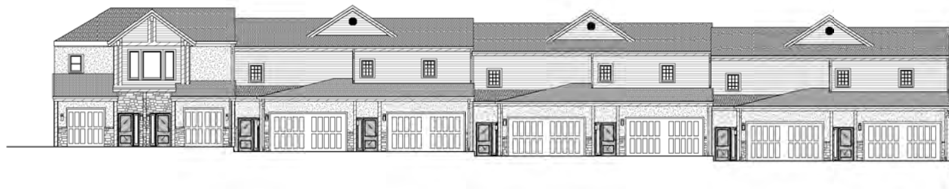
D1 NORTH ELEVATION BUILDING 5 A 1/8" = 1'-0"
