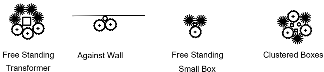
TYPICAL UTILITY BOX SCREENING DETAILS - NTS
