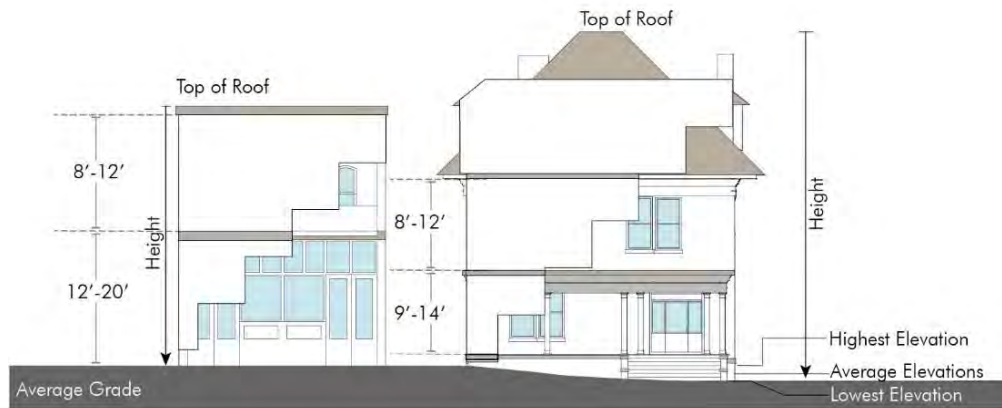
Figure 401-1 Building Height and Building Stories
