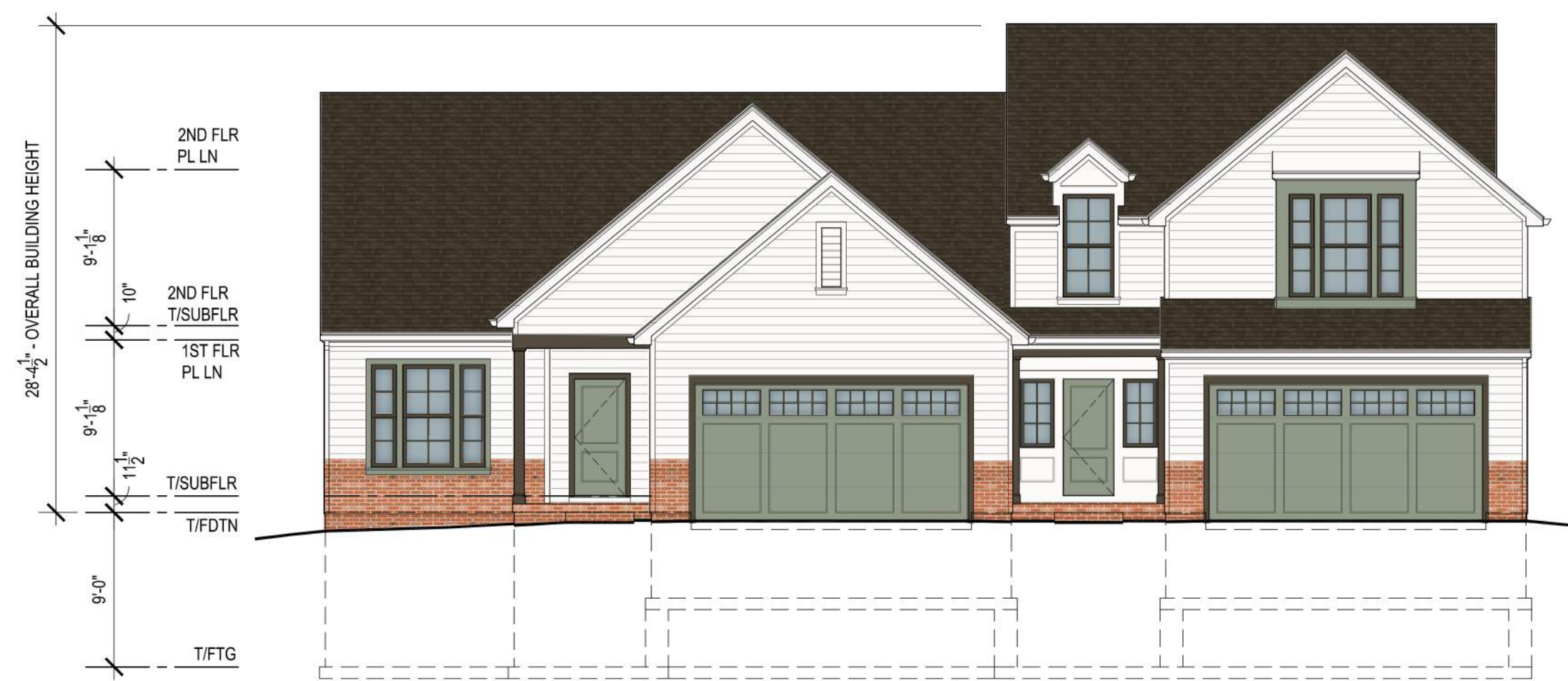
2 BUILDING ELEVATION TWIN VILLAS - FRONT ELEVATION 1/8" = 1'-0"
